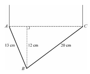
A rigid body *ABC* consists of two uniform rods *AB* and *BC*, rigidly joined at *B*. The lengths of *AB* and *BC* are 13 cm and 20 cm respectively, and their weights are 13 N and 20 N respectively. The distance of *B* from *AC* is 12 cm. The body hangs in equilibrium, with *AC* horizontal, from two vertical strings attached at *A* and *C*. Find the tension in each string.
