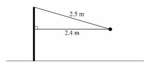
A ball of mass 0.08 kg is attached by two strings to a fixed vertical post. The strings have lengths 2.5 m and 2.4 m, as shown in the diagram. The ball moves in a horizontal circle, of radius 2.4 m, with constant speed v m s<sup>-1</sup>. Each string is taut and the lower string is horizontal. The modelling assumptions made are that both strings are light and inextensible, and that there is no air resistance.
