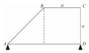
A uniform lamina ABCD has the shape of a square of side a adjoining a right-angled isosceles triangle whose equal sides are also of length a. The weight of the lamina is W. The lamina rests, in a vertical plane, on smooth supports at A and D, with AD horizontal (see diagram).
